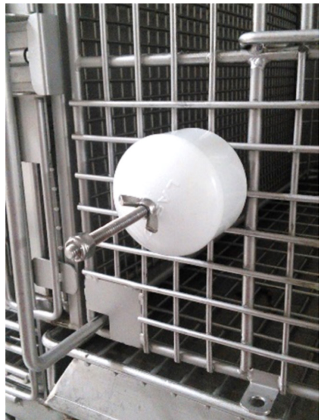
Figure 1. The browsing bowl device is attached to the cage front with 1-in. mesh.
