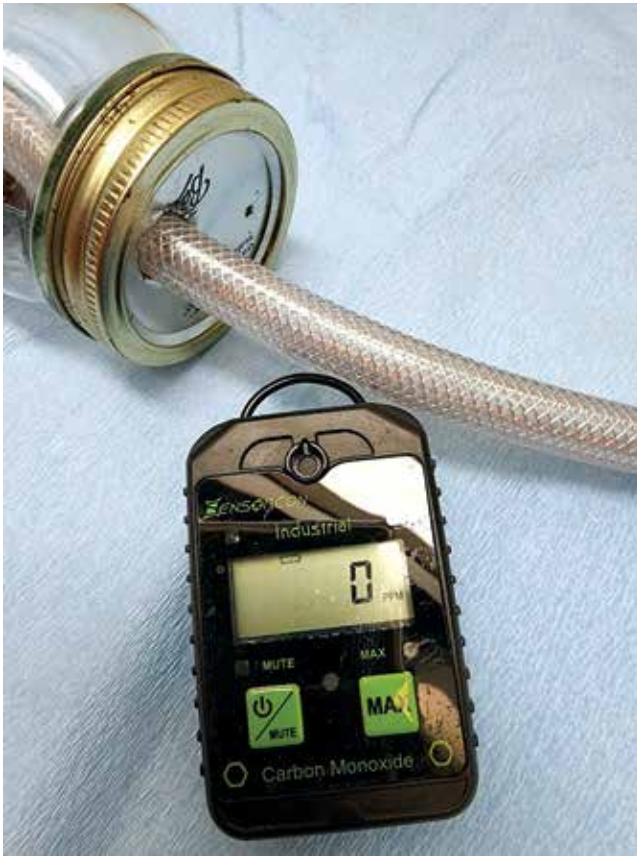
Figure 1. Experimental setup including clear glass pint jar with lid and CO meter.
