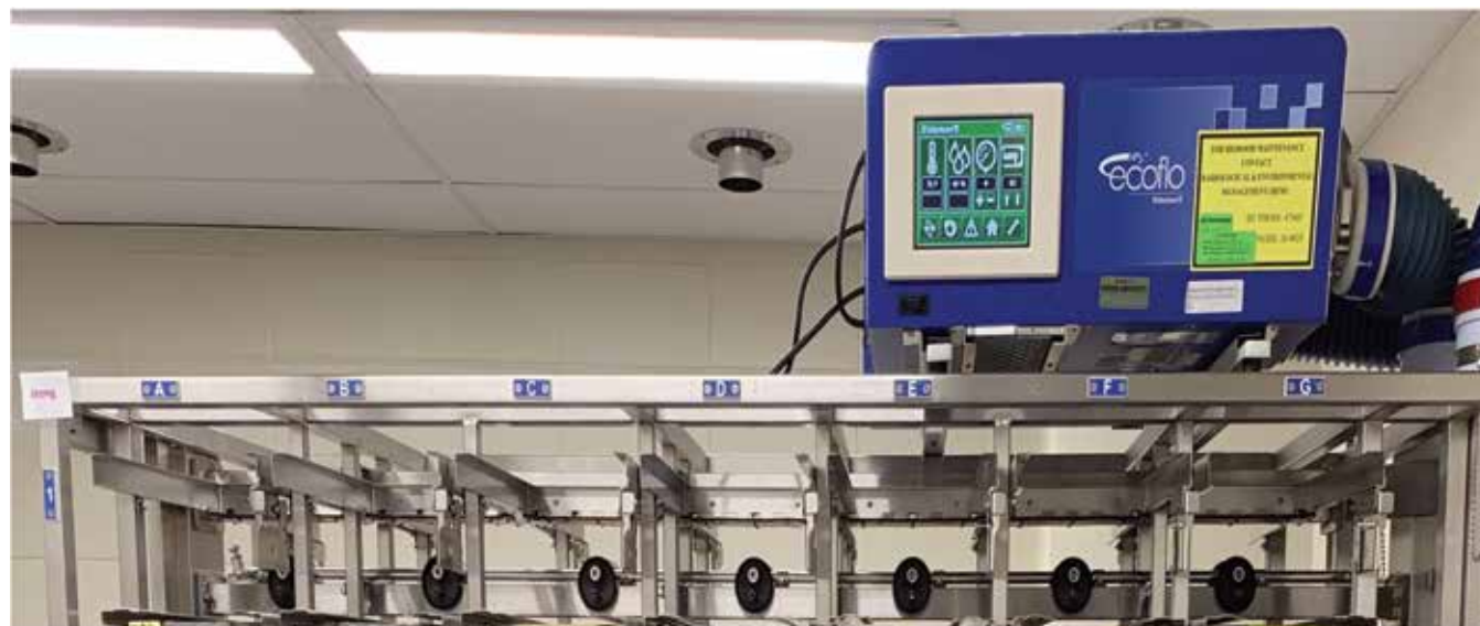
Figure 5. Visualization of the sampled locations across the top row of a ventilated rack to assess light variation.
