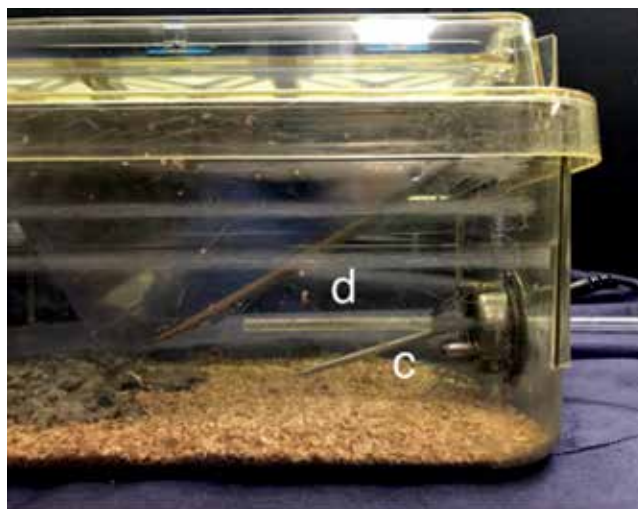
Figure 3. Side view of mouse cage showing the relative positions of the psychrometer probe (c) and gas-sampling tubing (d).
