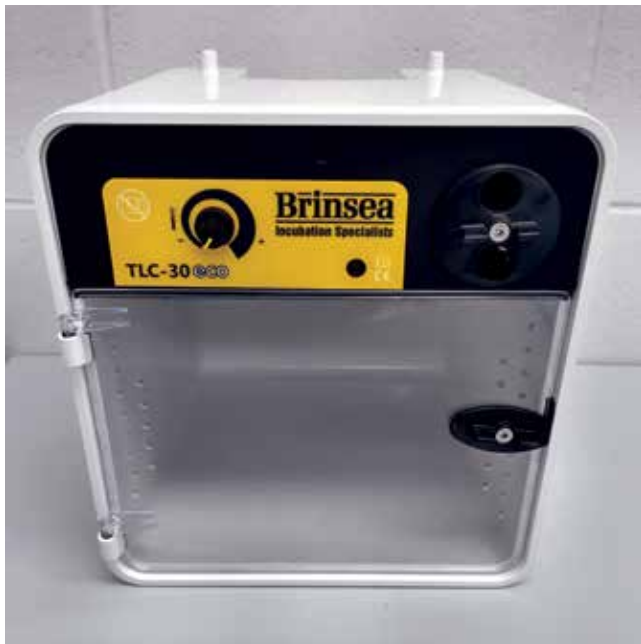
Figure 2. Small-animal forced-air incubator, front view, with temperature setting dial and manual air vent in the closed position to the left and right, respectively, on the front panel. Animals can be placed in the interior of the incubator by opening the clear, front-facing door.
