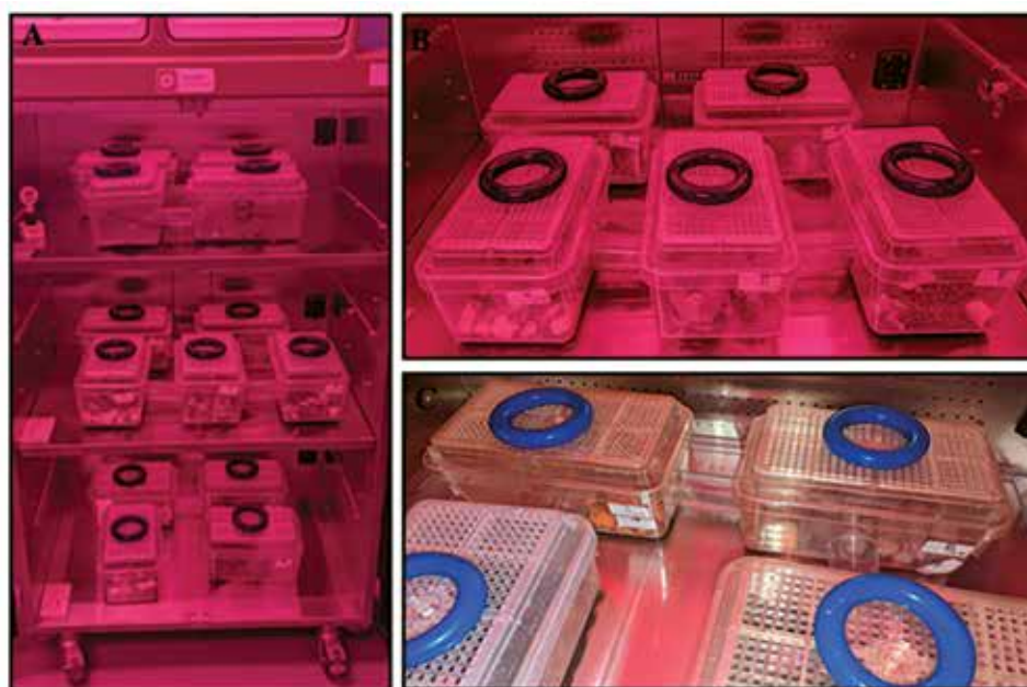
Figure 5. Tunnel systems with weights on lids. A) Multiple colonies housed in Tecniplast Aria Ventilated Cabinet BIO-36; B) 5-tunnel caging system; C) 4-cage tunnel system.
