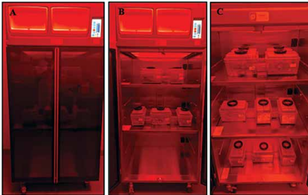
Figure 2. Tecniplast Aria Ventilated Cabinet BIO-C36 in a housing room. A) Closed cabinet; B) 2 Colony caging placed in temperature-controlled unit; C) Multiple colonies housed on 3 shelves in a ventilated cabinet.
