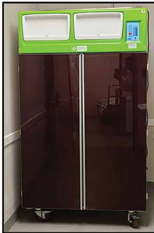
Figure 1. Tecniplast Aria Ventilated Cabinet BIO-36 in a housing room.
