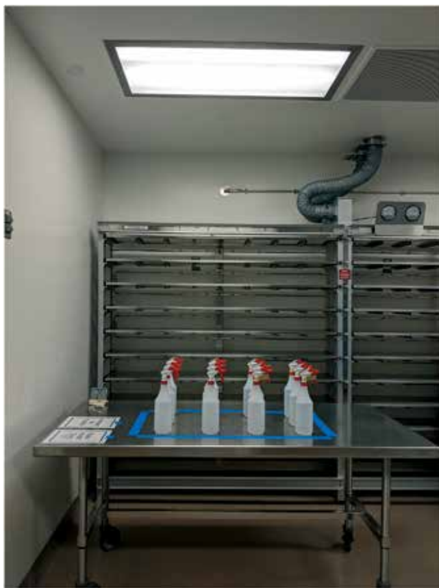
Figure 2. Set-up of the table and bottles within the empty rodent housing room. Twelve bottles (3 rows by 4 columns) were positioned at the center of a stainless-steel table, approximately 1 m tall, directly below the lighting banister. The exact positioning was adjusted until all bottles were exposed to the same average light intensity (lux), as confirmed by a light meter.
