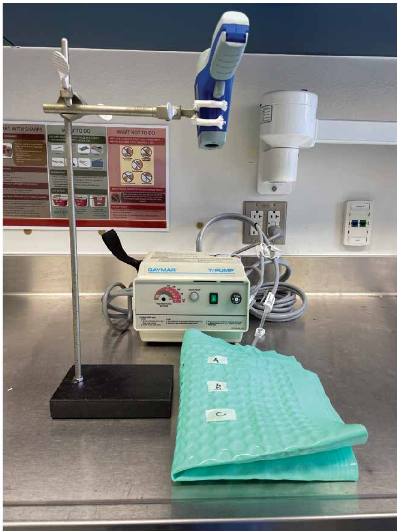
Figure 1. Photo depicts circulating warm water blanket and pump set up. Locations A, B and C are listed on the water blanket. Infrared gun and holding apparatus depicted adjacent to the blanket.
