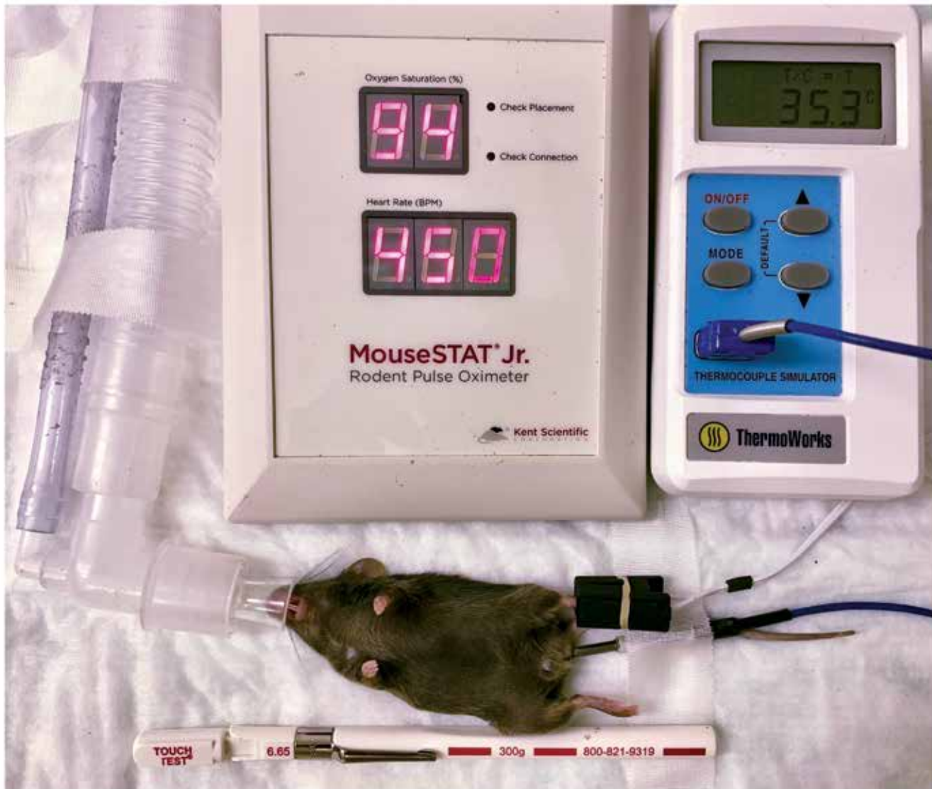
Figure 1. Mouse anesthetized and instrumented for physiologic monitoring. The face mask provides supplemental oxygen, and SpO 2 and HR are measured using a mouse-specific pulse oximeter. Temperature is measured using a rectal temperature probe and thermal support was provided by a circulating water blanket and heat lamp. Paw withdrawal reflex was obtained by application of a 300-gram Touch Test device.
