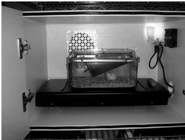
Figure 1. Experimental setting for thermoregulation and locomotor activity studies at UAMS showing a standard static home cage, 4W light to establish a photoperiod within the experimental space (upper right), exhaust fan (next to the light), and warm air heating vent to manipulate ambient temperature within the experimental space (upper left).
