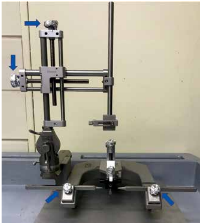
Figure 3. A stereotaxic apparatus with aluminum foil applied to adjustment knobs. The blue arrows indicate the 4 knob locations sampled in this study.
