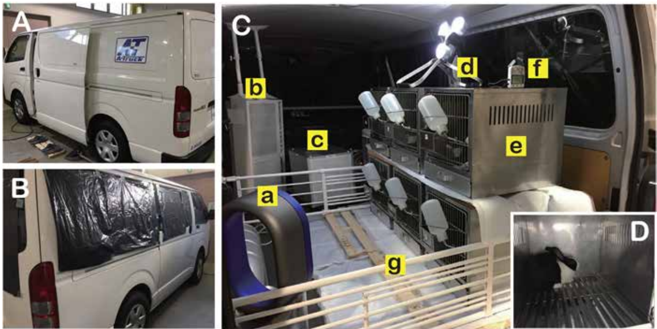
Figure 1. The cargo van system provides environmentally stable, short-term housing for laboratory rabbits. (A) Refrigerated cargo van. (B) Standard cargo van with black plastic sheets. (C) Interior of the cargo van equipped with a humidifier (a), air conditioner (b), photocatalyst deodorizer (c), LED lamp (d), rabbit cage (e), data logger (f), and fence (g). (D) The inside of a rabbit cage.
