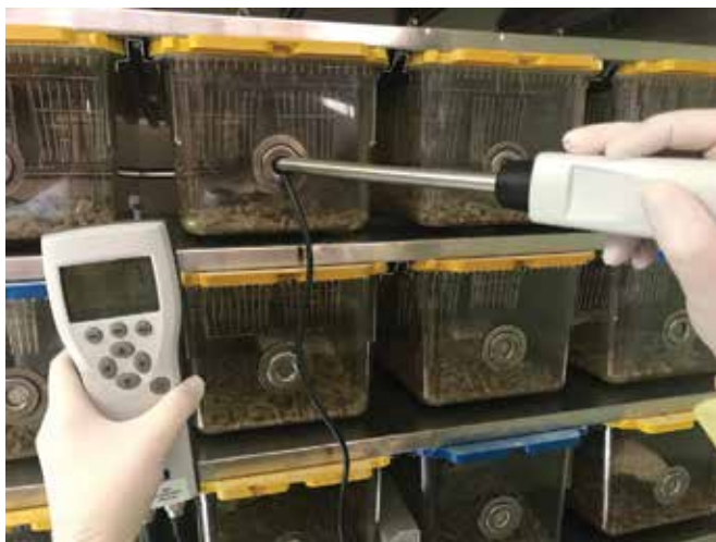
Figure 2. The intracage environment was assayed by using 2 sensitive instruments whose sampling probes were inserted into the cage through the grommet opening. Assays were made just prior to and just after cage change or scoop.
