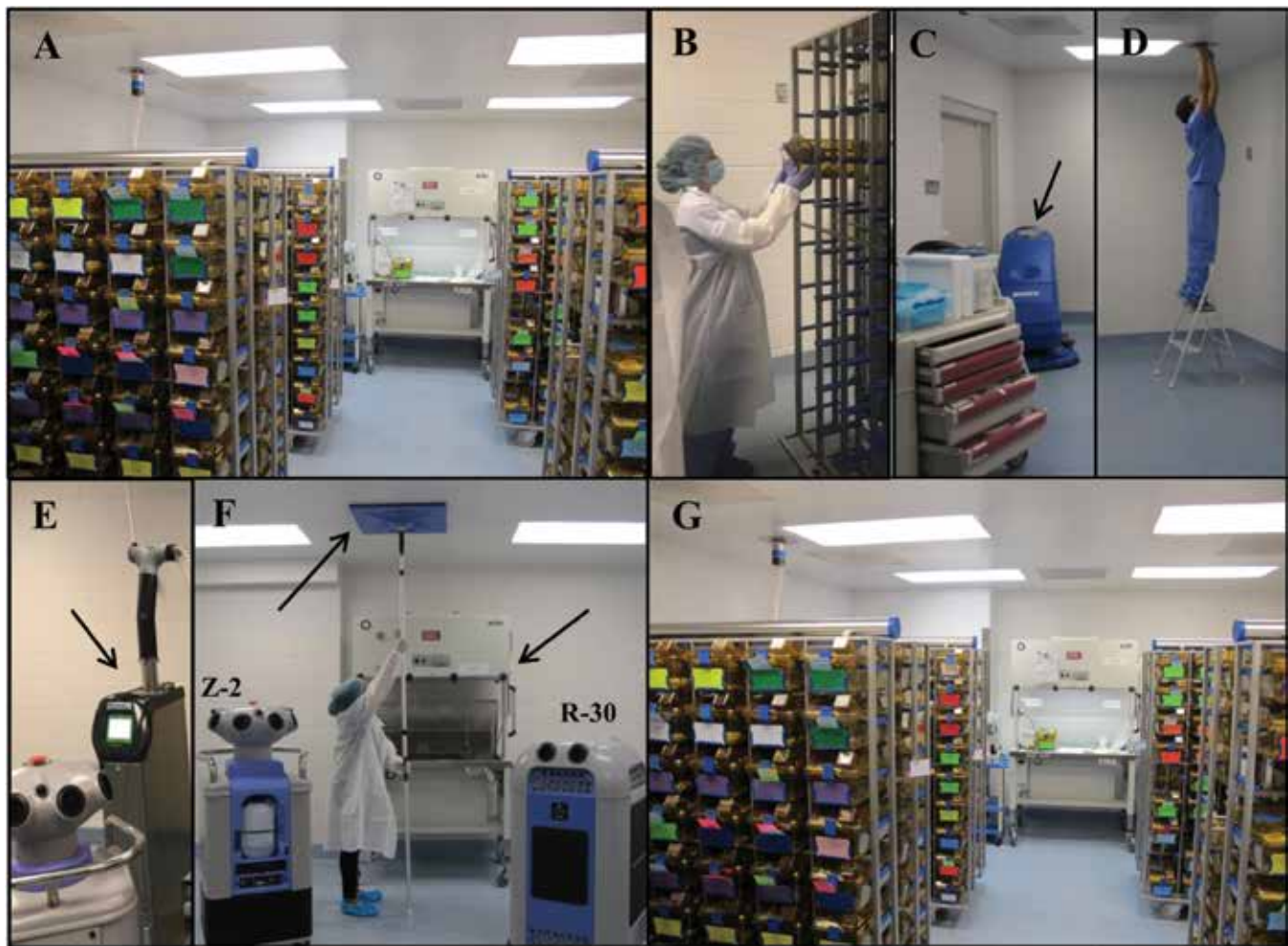
Figure 4. (A) The housing room scheduled for VHP decontamination, from which occupied IVC racks were taken to the flex room, where occupied IVC were transferred to (B) VHP-sterilized racks. (C) In the now unoccupied housing room, storage unit drawers were opened, the floor scrubber was run (arrow), (D) thimbles were covered, (E) VHP-sterilized AHU with hoses were positioned (arrow), (F) HVAC supply and exhaust vents were covered (left arrow) and animal transfer stations were left powered on (right arrow), and the Z2 generator and R30 accelerator were positioned. (G) The next morning, murine occupied IVC racks were brought from the flex room to the VHP-decontaminated housing room and connected to AHU.
