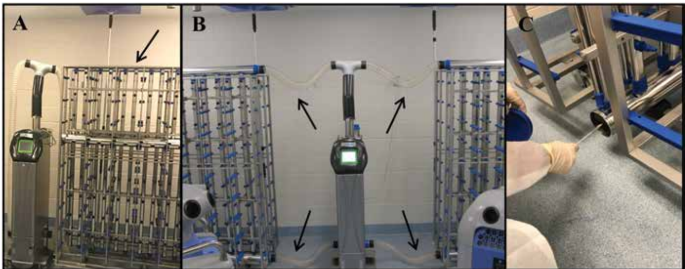
Figure 2. (A) IVC racks and AHU were VHP decontaminated during months 1 through 5 in the static–open setting, such that AHU were off, hoses were disconnected, and rack plenums were unassembled (arrows). (B) In contrast, during months 6 through 12, IVC racks and AHU were VHP exposed in the active–closed setting, with IVC rack plenums assembled, sealed, and hoses connected (arrows) to AHU set to the VHP cycle. (C) Airways (here an exhaust plenum) were sampled either when soiled, after they were washed, or after VHP exposure by using a sterile swab to trace a circular pattern for 3 circumferences as the tip was rolled. Sample-bearing swabs then were assessed by using C. bovis PCR analysis.
