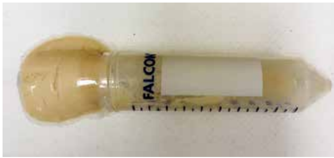
Figure 2. LEN has congealed within the tube within 24 h; flow through the sipper tube was obstructed.
