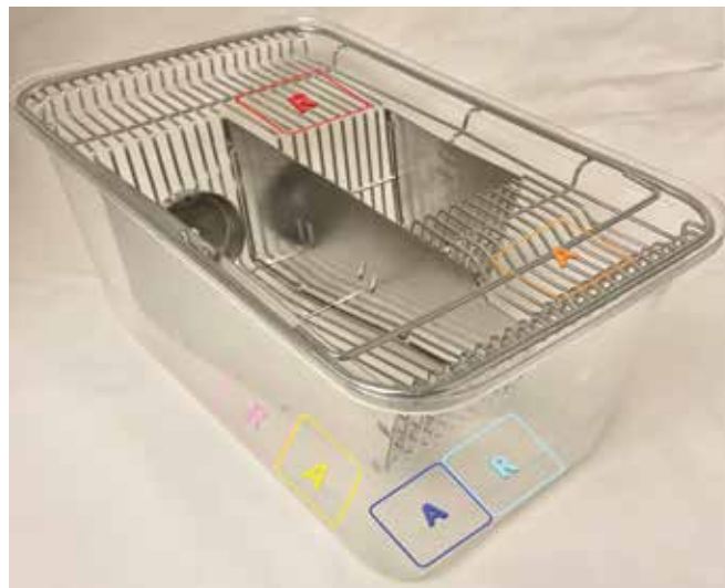
Figure 1. Sampling locations (10 cm 2 rectangles) were drawn onto the outside of each cage by using a wax pencil. Samples were obtained from the cage side (pink and yellow boxes), cage floor (dark and light blue boxes), and underside of the wire top (orange and red boxes). A, ATP swabs; R, RODAC plates.
