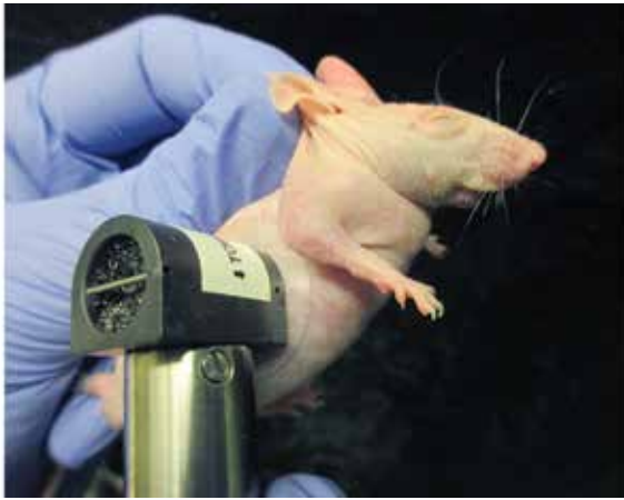
Figure 1. SCID mouse restrained for placement of the TEWL Probe. The TEWL probe contains paired sensors that measure humidity and temperature and computes 2 separate vapor pressures; the difference between the vapor pressures at the 2 points is used to calculate evaporative water loss from the skin. Restraint time is \leq 30 s.
