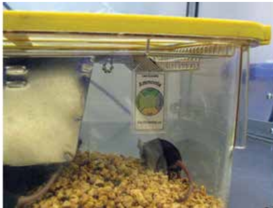
Figure 1. Ammonia sensor suspended from wire top within a mouse cage. The central disk is a light-green color, designated by the number 2, indicating an intermediate (1–25 ppm) ammonia level.
