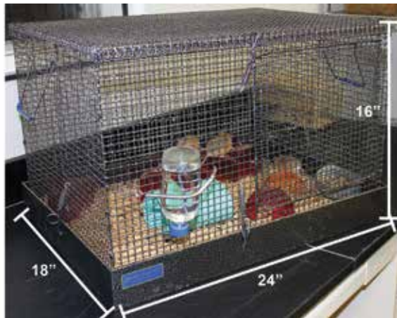
Figure 3. Wire cages used for housing the A. cahirinus colony at our institution. Cages (width, 24 in.; height, 18 in.; depth, 16 in.; Quality Cage Company, Portland, OR) are made from 1/4-in. galvanized-steel wire and can be disassembled for processing through a cage washer. The wire sides and top provide excellent enrichment.
