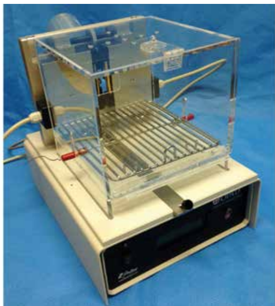
Figure 1. Orofacial pain assessment device. A rat is placed in the test box with access to a reward bottle filled with diluted sweetened condensed milk. To access the reward sipper tube, the rat must make facial contact with 2 parallel vertical metal thermodes which can be adjusted to contact the same shaved area of the face each test session. The temperature of the metal thermodes are controlled by a computer. The number of facial contacts with the metal thermodes and the number of licks to the sipper tube are counted by the computer. The nontraumatic nature of the assay allows the same rat to be evaluated multiple times.
