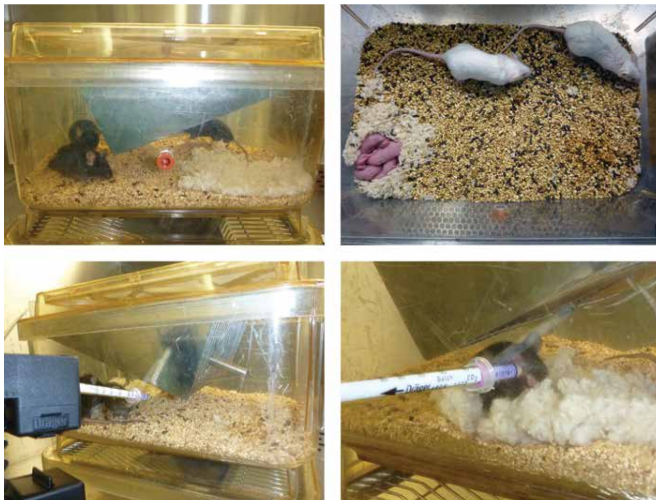
Figure 1. Cage modifications were made to accommodate gas level measurements. Representative pictures depict a closed cage from the outside (upper left), an open cage from the inside (upper right), and closed cages during gas measurements (lower left and right).
