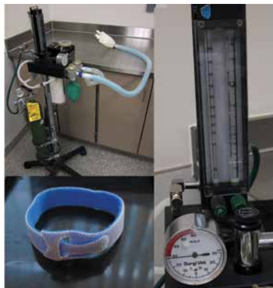
Figure 1. Pressure test apparatus. An anesthetic machine was arranged with an F-circuit and a 0.5-L breathing bag, and the pop-off valve was closed. The circuit was pressure-tested to ensure there were no leaks in the system. The bottom 5 cm of the glove cuff was stretched tightly around the end of the breathing circuit and secured tightly by using a hook-and-loop cable tie, with the loop side against the glove.
