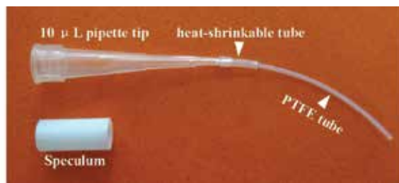
Figure 1. Transcervical embryo transfer device for mice.
