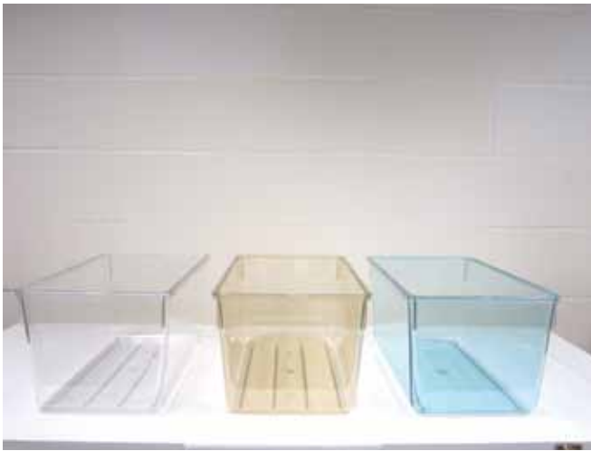
Figure 1. Photoimage showing the standard polycarbonate translucent clear (left), polysulfone amber (center), and polycarbonate blue (right) rat cages. All animal cages had the same dimensions (19 in. × 10.5 in. × 8 in.; wall thickness, 0.1 in.) and were autoclavable to 121 °C.
