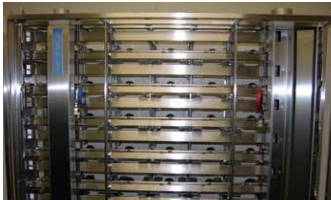
Figure 2. View of the backside of the IVC rack, indicating the location of the supply and exhaust vertical plenum covers. The blue-labeled supply cover (left) is closed; the exhaust cover (right) is open, revealing the location of the shelf horizontal exhaust manifolds.
