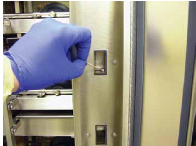
Figure 3. Close up of shelf horizontal exhaust manifold during sampling.
