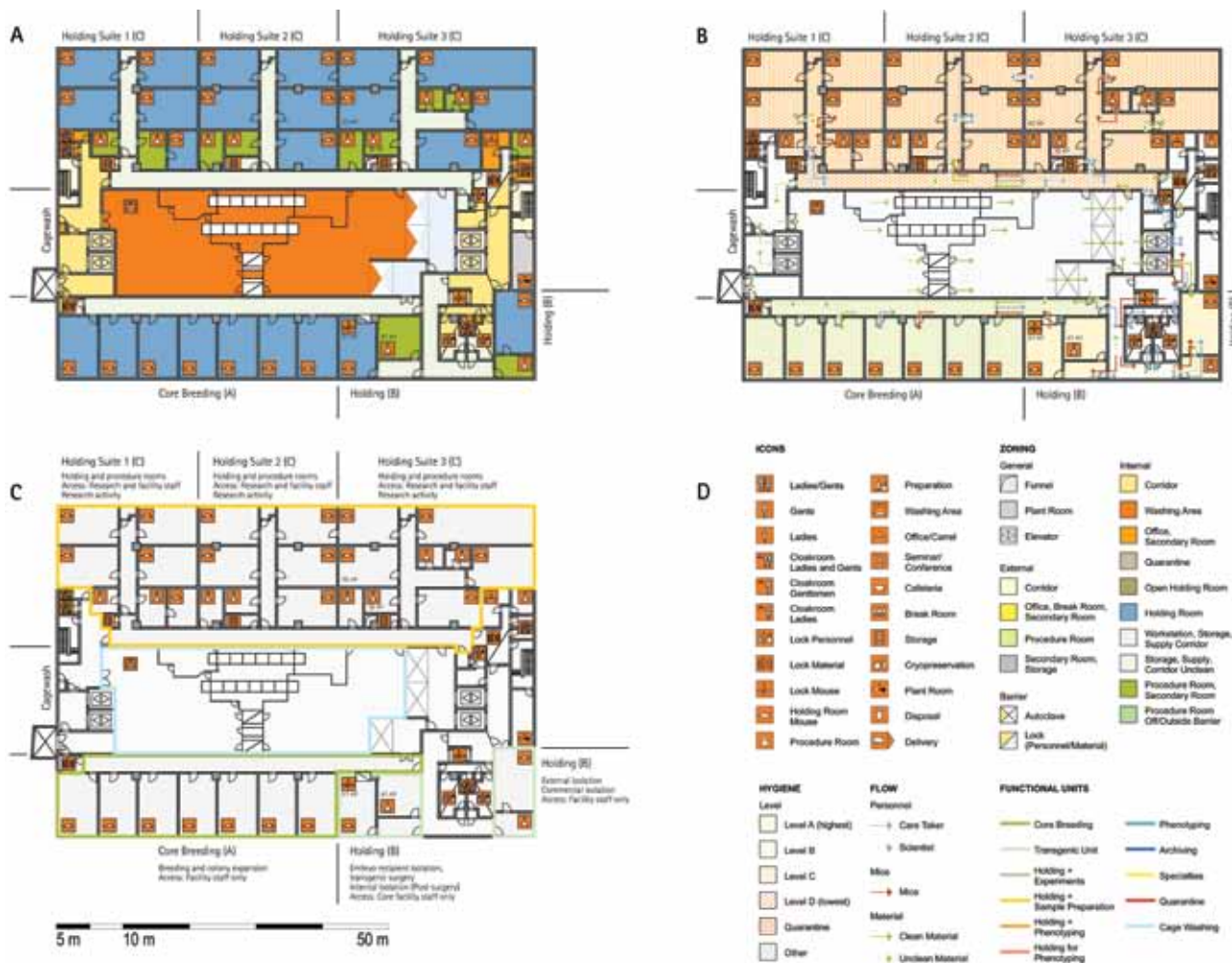
Figure 1. Schematic floor plans—facility 1, plan 1. Three types of schematic floor plans that outline the layout of the rooms and floors, the hygiene zones, and traffic flow were generated from the information collected at the visited facilities. (A) Zoning scheme. The zoning scheme shows the various functional types of rooms, which are represented by icons. In addition, color coding indicates areas outside and within the barrier as well as the various functional units. (B) Flow and hygiene levels scheme shows the flow of personnel (caretaker, scientists), mice, and material (clean and soiled) and the various hygiene levels. (C) Functional unit scheme. Details of the functional use of the various units and access of the facility staff and scientists are presented. (D) Description of the icons and colors used in the various floor plans.
