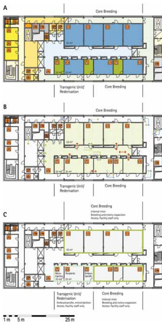
Figure 11. Schematic floor plans—facility 4, plan 2. (A) Zoning scheme. (B) Flow and hygiene levels scheme. (C) Functional unit scheme. For a description of the icons and colors used in the floor plans, see the legend to Figure 1.
