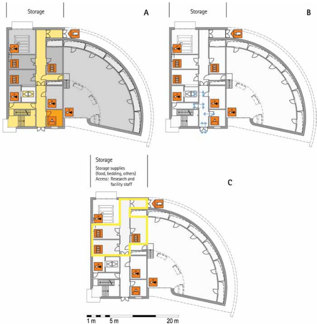
Figure 16. Schematic floor plans—facility 4, plan 7. (A) Zoning scheme. (B) Flow and hygiene levels scheme. (C) Functional unit scheme. For a description of the icons and colors used in the floor plans, see the legend to Figure 1.
