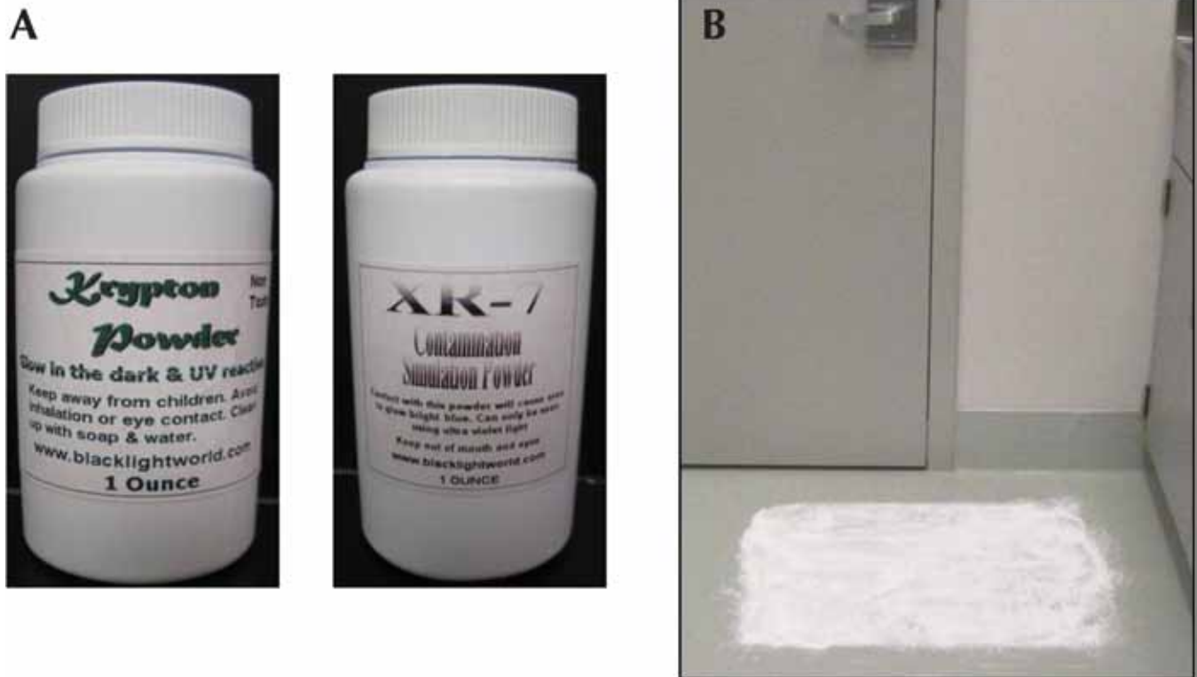
Figure 2. (A) Krypton and XR7 contamination powder. (B) A thin layer (1 oz) of XR7 powder applied to the floor inside of the animal room door. Powders appear white in UV light.
