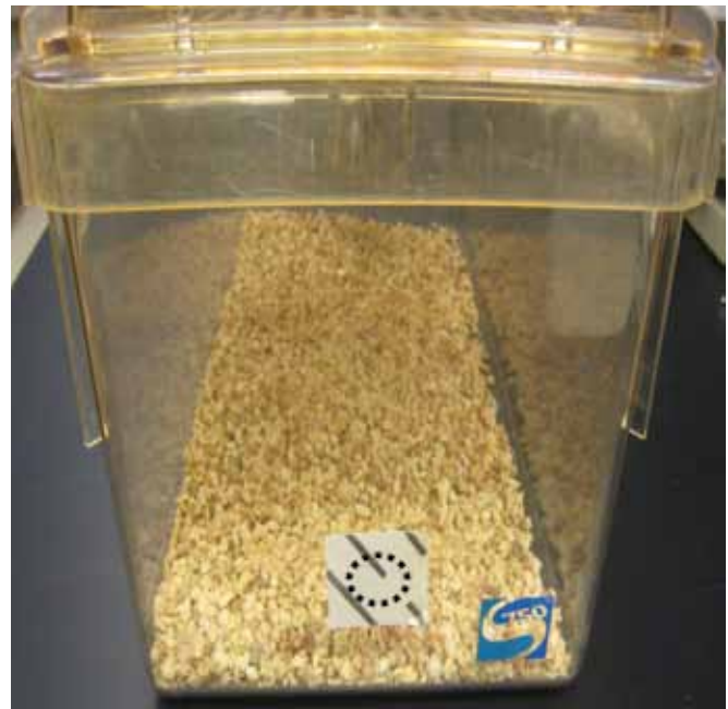
Figure 1. Cage modification. A 1/4-in.-diameter hole was drilled in the front of a microisolation mouse cage, 4 cm from the cage bottom. Dotted line indicates location of hole in cage wall.
