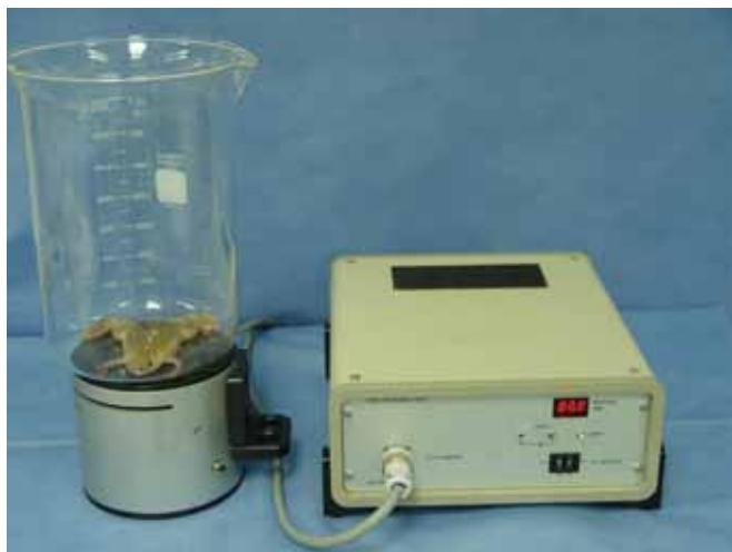
Figure 1. Photograph of the testing mechanism, including the Hargreaves apparatus, glass chamber, and Xenopus laevis .
