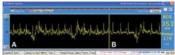
Figure 5. Mouse ECG recordings inside a 11.7-T magnetic field (A) with and (B) without imaging gradients, showing increased noise during gradient switching but good R wave detectability.
