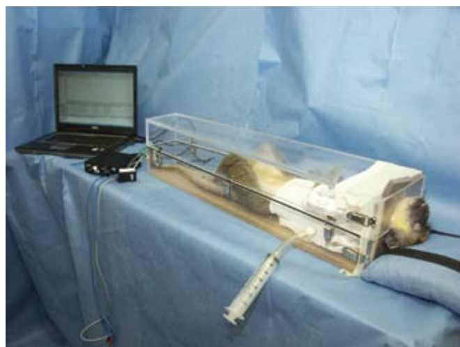
Figure 1. African green monkey fitted with a nonrestraining protective jacket and positioned in a medium plethysmography box.
