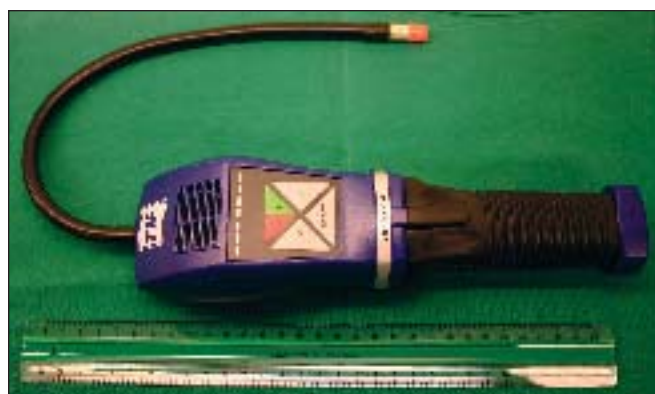
Figure 2. The leak detector for halogenated gas refrigerants.
