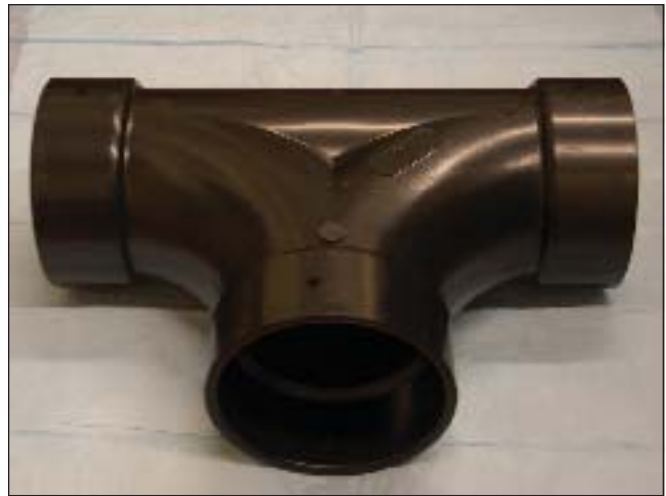
Figure 2. Acrylonitrile-butadiene-styrene (ABS) refuge pipes added to tanks A and B, December 31, 2003.
