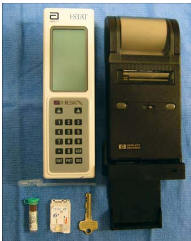
Figure 1. Equipment needed for collection and processing of whole-blood samples: a lithium heparin (green-topped) 1.3-ml tube, a disposable plastic pipette, the E6+ Mini-Urgent Care cartridge, the i-STAT portable clinical analyzer, and an infrared printer. The standard-size office key is provided for scale.
