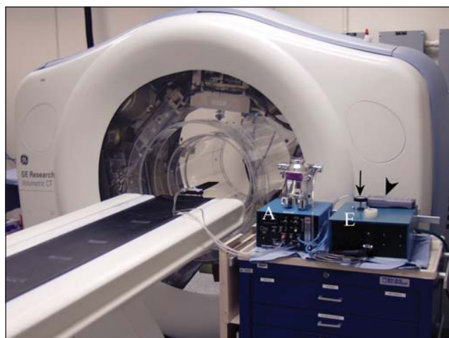
Figure 1. Prototype flat-panel computed tomographic scanner set up with small-animal ventilator (A), electronic breath-hold device (E), adjustable pressure regulator (arrow), and pressure manometer (arrowhead).
