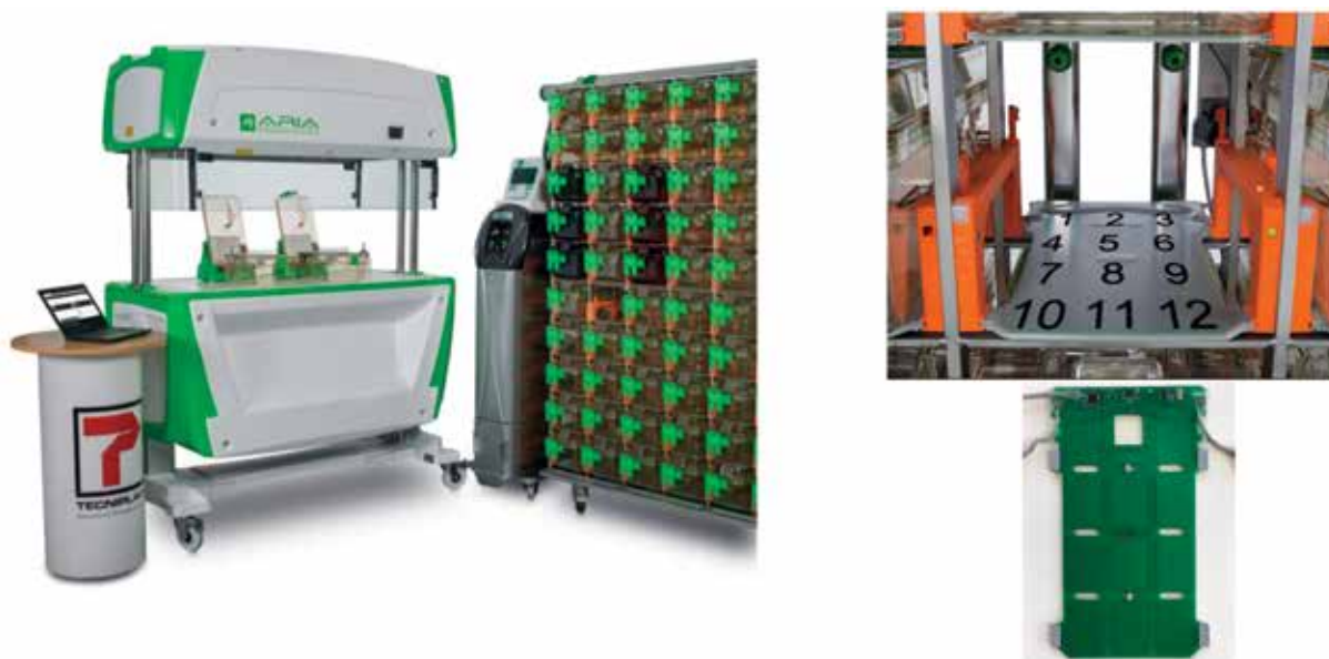
Figure 1. The digital ventilated cage system is an automated home-cage monitoring that continuously records spontaneous activity in the cages. The system can collect data from thousands of home cages simultaneously.
