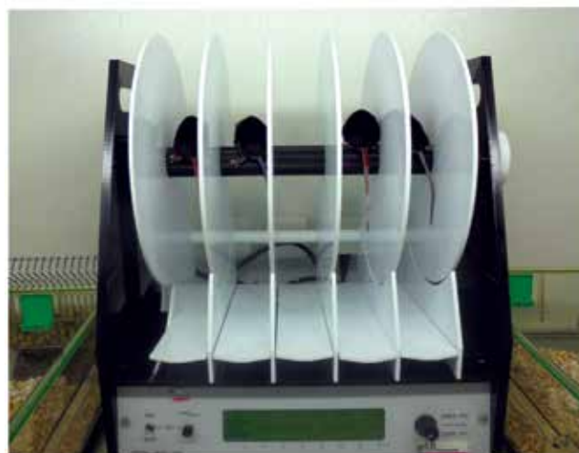
Figure 2. The rotarod test is based on a gradual and continued acceleration of a rotating rod onto which mice are placed. Data collected corresponds to the riding time (the amount of time each mouse stays on the rod before falling off or a passive rotation) and the speed (from 4 to 40 rpm).
