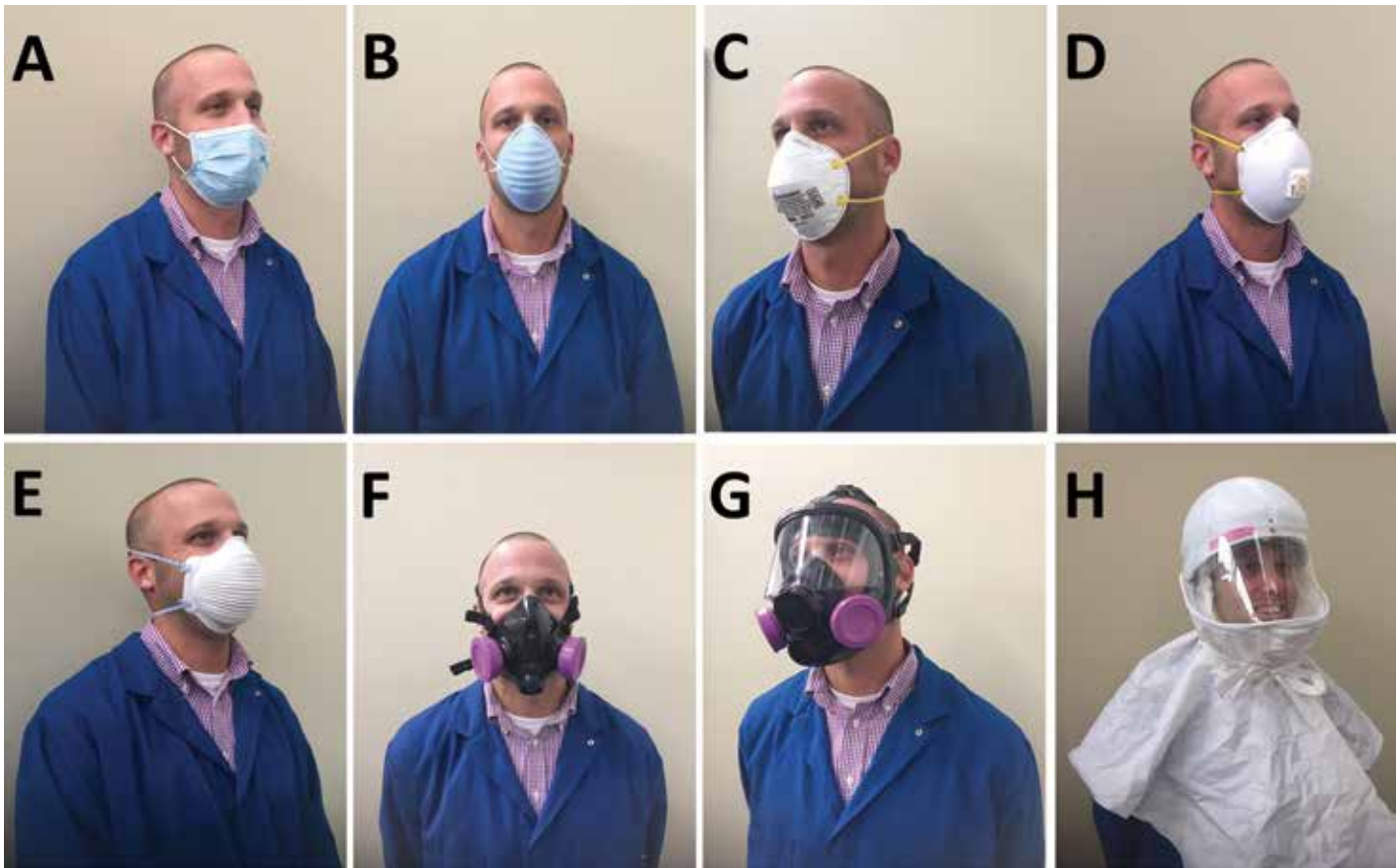
Figure 4. Masks and respirators. (A) Three-pleated surgical mask. (B) Surgical molded mask. (C and D) N95 respirators with a metal band that seals the nose bridge area. Note: on a high nose arch or a thin nose, the metal band does not work well and may interfere with fit tests. (E) Flexible-fit design N95 respirator offers a pinch-free molded nose bridge for facial features that may not fit well with other models. (F) Half-facepiece respirator with HEPA filter cartridge. (G) Full-facepiece respirator with HEPA filter cartridge. (H) Powered air-purifying respirator (PAPR) with HEPA filter cartridge within helmet.
