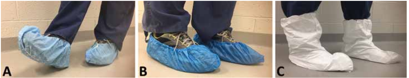
Figure 3. Shoe and boot covers made of (A) polypropylene with nonskid soles, (B) polyethylene, and (C) flash-spun high-density polyethylene.
