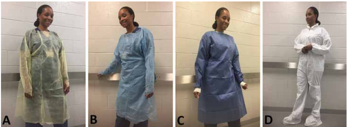
Figure 2. Protective apparel. (A) Spunbond multiply polypropylene gown; (B) apron-style polyethylene gown. Because the polypropylene gown offers only basic protection and the polyethylene gown has an open back, neither meets the PB70 standard for isolation gowns. (C) Surgical gown made of multilayered (spunbonded-meltblown-spunbonded) fabric. (D) Flash-spun, high-density polyethylene (“Tyvek”) suit.
