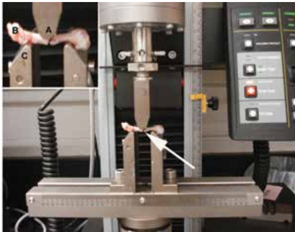
Figure 3. Image of the right femur after breaking, demonstrating the position of the external supporting pins, fracture through the lesion, and the break on the tension surface (convex side) first. The arrow in the main figure shows the lesion with the break; and the inset shows the (A) upper anvil, (B) right femur, and (C) lower supporting pins.
