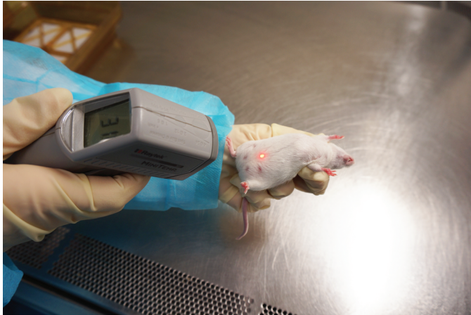
Figure 1. The infrared thermometer (MiniTemp MT4, Raytek, Santa Cruz, CA) and demonstration of the method used to record BT.
