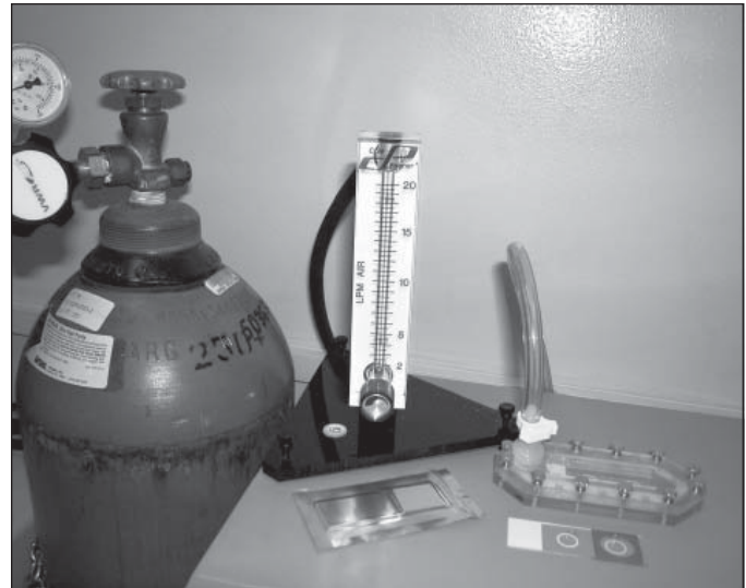
Figure 1. Evaporative drying system for sperm. Compressed ultrapure nitrogen gas is blown through a regulator and flow meter, into the drying chamber, and out through a hole at the right end of the drying chamber. A glass slide with 2 10-mm circular areas and a silicone isolator and a sperm sample vacuum-sealed in a metallized nylon bag also are shown.
