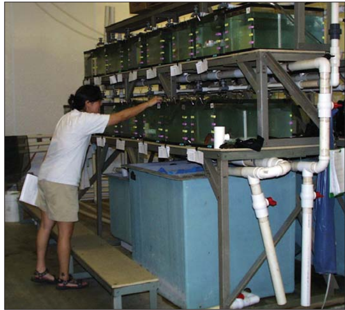
Figure 1. Racks of individual fish tanks on a shared recirculating system.
