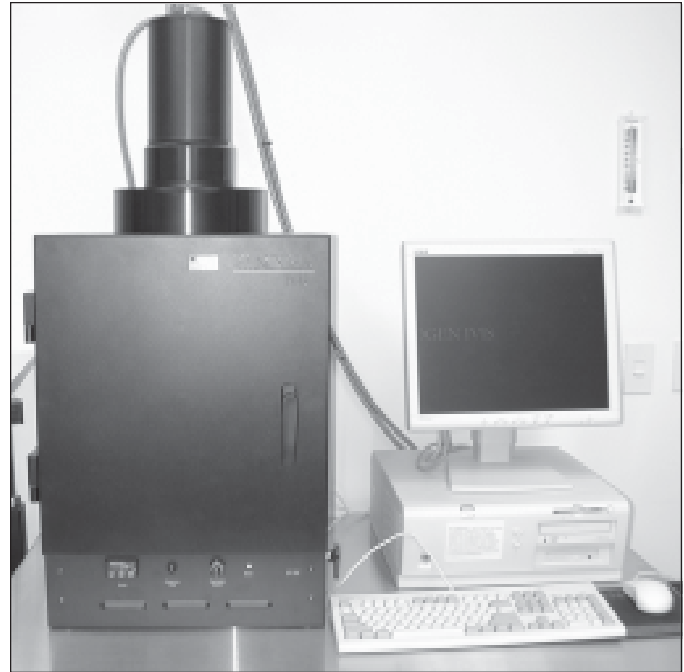
Figure 2. An imaging system consists of a light-tight box where animals are placed, the cooled charge-coupled device camera to detect light, and image processing software.
