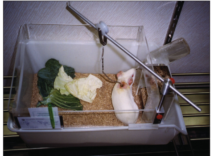
Figure 1. Photograph of a conscious, long term-cannulated guinea pig in its modified housing, using a gimbal device to support the cannulae. The spring coil encases and protects the cannulae, which exit from the nape of the neck. The spring coil is attached to a roller on the crane-like arm that allows the instrumented guinea pig full range of movement around the housing.
