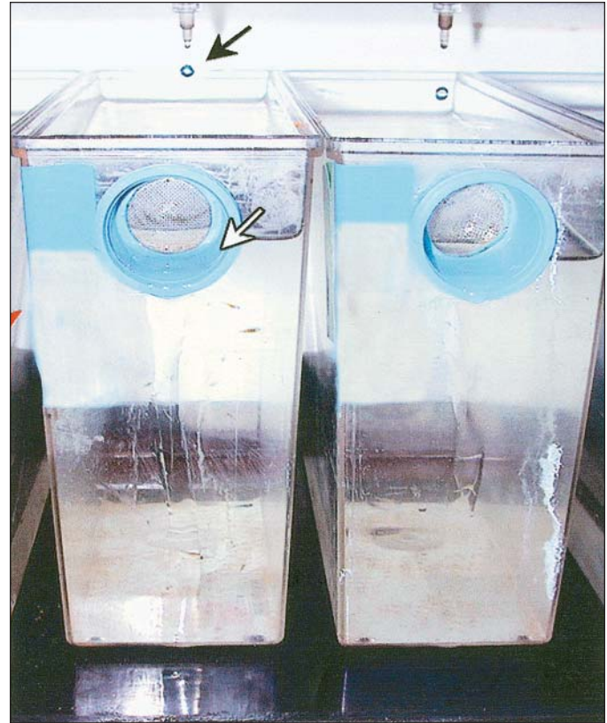
Figure 1. Photograph of representative zebrafish housing units used at this research laboratory and available through a commercial vendor. Fry were reared in individual 1- to 4-L capacity units. Water exchange occurs through afferent fresh water (black arrow) from above, with effluent draining through a mesh screen-covered orifice in the front of the unit (white arrow).
